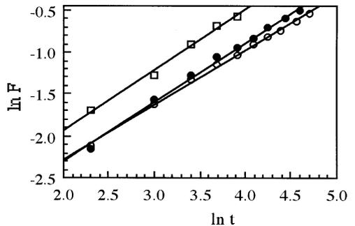
Figure 6. Swelling kinetics curves of AAm/MA hydrogel in the solution of tryptophan at various pH.
