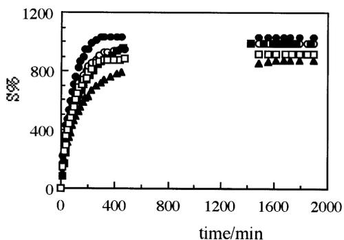
Figure 1. The influence of pH on the swelling behaviour of AAm/MA hydrogel in the buffer solution.
