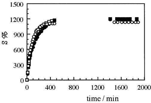
Figure 3. The swelling curves of AAm/MA hydrogel in the buffer solutions at the pH values of amino acids.
