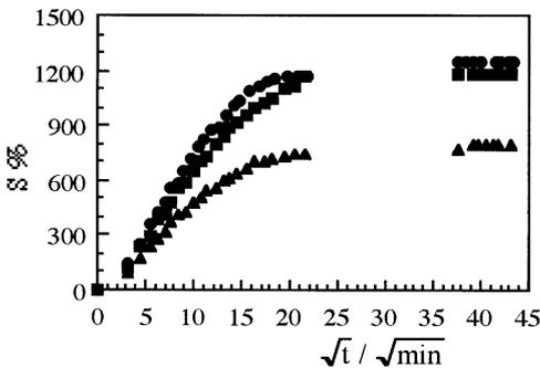
Figure 5. Swelling rate curves of AAm/MA hydrogel in the solution of tryptophan at various pH.
