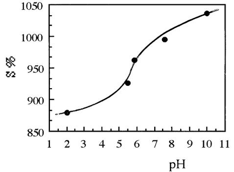
Figure 4. The change of the equilibrium swelling of AAm/MA hydrogel with pH in the buffer solution.
