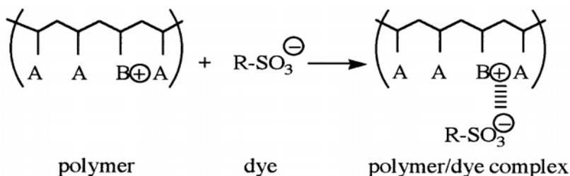
Scheme-3. Ion/ion interaction between negative charge of sulfonyl group on the anionic dye and positive charge of polymer.
