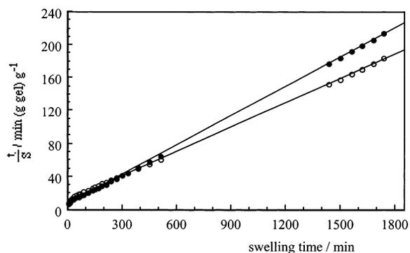
Fig. 3. Swelling kinetics curves of HEMA/AAm hydrogel containing 89.58% AAm: ●, water; ○, nutrient medium.
