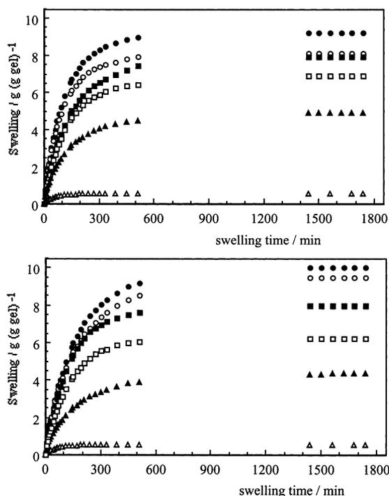
Fig. 2. (a) Swelling curves of HEMA/AAm hydrogels in water: ●, 100% AAm; ○, 89.58% AAm; ■, 81.09% AAm, □, 74.17% AAm; ▲, 63.18% AAm, △, 0% AAm. (b) Swelling curves of HEMA/AAm hydrogels in the nutrient medium: ●, 100% AAm; ○, 89.58% AAm; ■, 81.09% AAm, □, 74.17% AAm; ▲, 63.18% AAm, △, 0% AAm.
