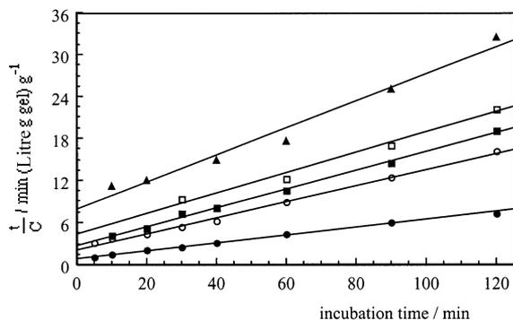
Fig. 7. Ethyl alcohol production kinetics curves of immobilized *S. cerevisiae* in the HEMA/AAm hydrogels: ●, 100% AAm; ○, 89.58% AAm; ■, 81.09% AAm, □, 74.17% AAm; ▲, 63.18% AAm.
