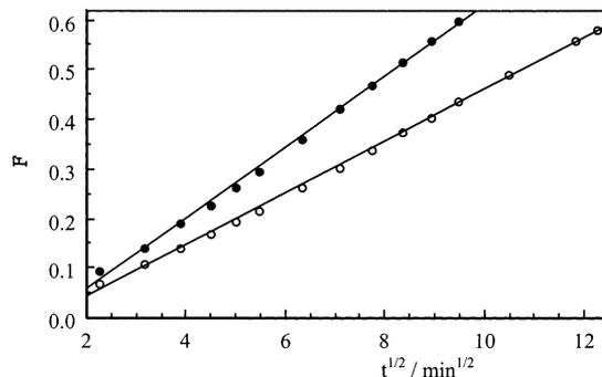
Fig. 5.  $F$ – $vt$  curves of HEMA/AAm hydrogels containing 89.58% AAm: ●, water; ○, nutrient medium.
