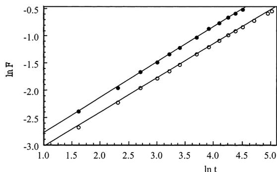
Fig. 4.  $\ln F$ – $\ln t$  curves of HEMA/AAm hydrogel containing 89.58% AAm: ●, water; ○, nutrient medium.
