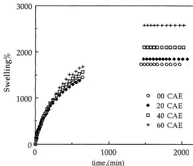
Fig. 1. Swelling isotherms of poly(AAm-co-CA) hydrogels crosslinked by EGDMA.
