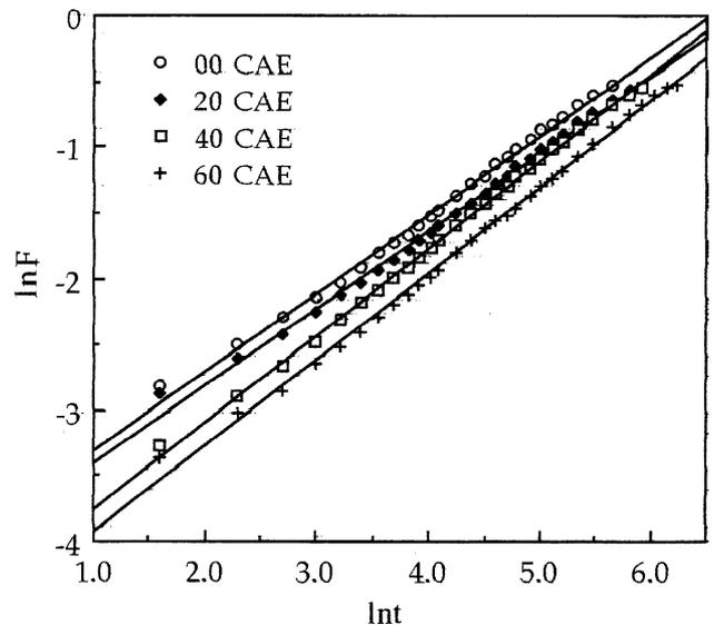
Fig. 3. Swelling kinetics curves of poly (AAm-co-CA) hydrogels crosslinked by EGDMA.
