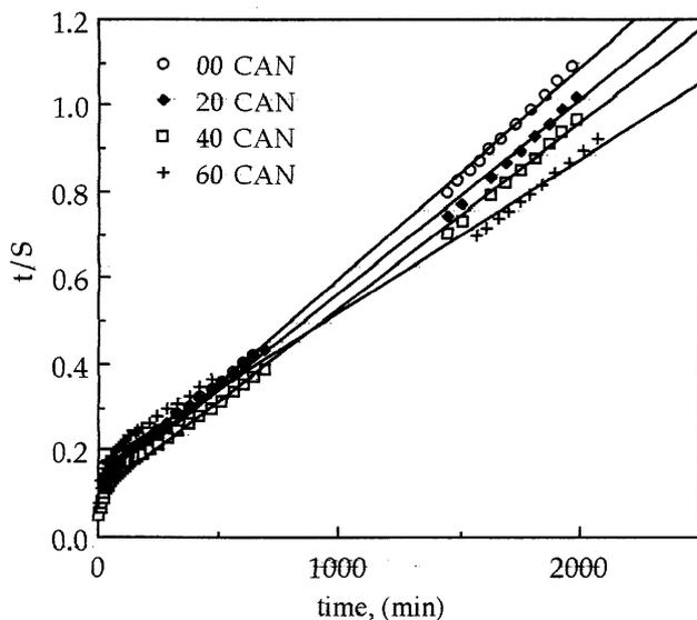
Fig. 2. Swelling rate curves of poly(AAm-co-CA) hydrogels crosslinked by NMBA.
