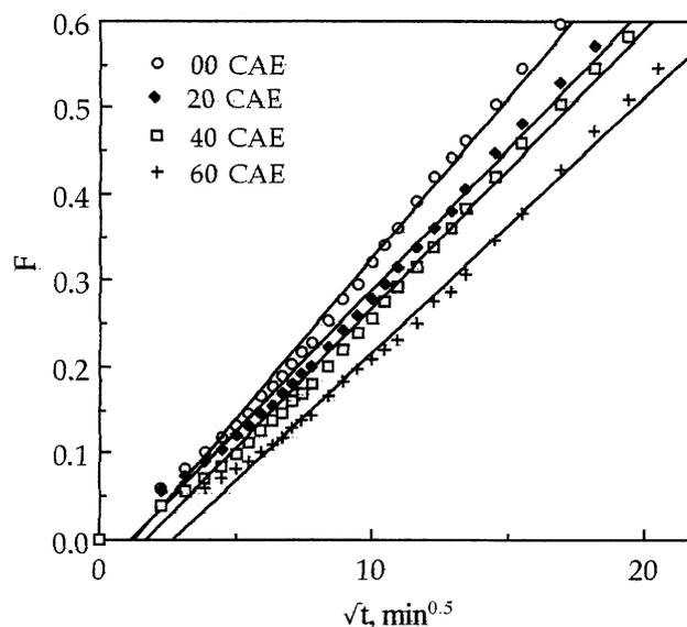
Fig. 4. Diffusion curves of poly (AAm-co-CA) hydrogels crosslinked by EGDMA.
