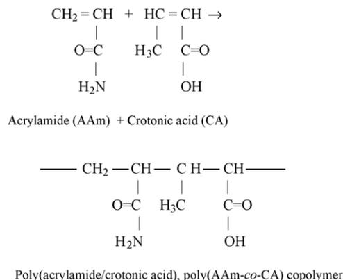
Fig. 2. Chemical structures of monomers and possible binding mechanism between acrylamide and crotonic acid for crosslinked poly(AAm-co-CA) copolymers.
