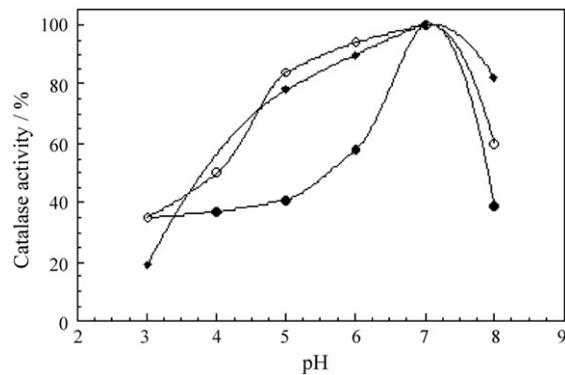
Fig. 7. pH profiles of catalase: (●) CB-Ch-CAT, (○) Ch-CAT and (◆) CAT (activities were assayed at 35 °C by using 10 mM H<sub>2</sub>O<sub>2</sub> prepared in appropriate buffer solution).
