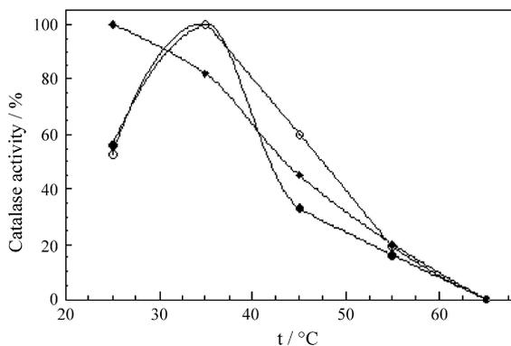
Fig. 8. Thermal stability of catalase: (●) CB-Ch-CAT, (○) Ch-CAT and (◆) CAT (after incubation at indicated temperature, activities were assayed at 35 °C by using 10 mM H<sub>2</sub>O<sub>2</sub> prepared in 50 mM phosphate buffer at pH 7.0).
