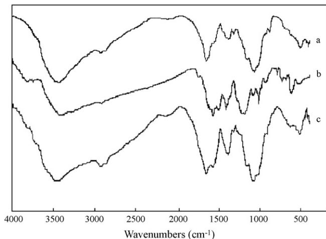
Fig. 4. FTIR spectra of Ch-bead (a), CB (b) and CB-Ch-bead (c).
