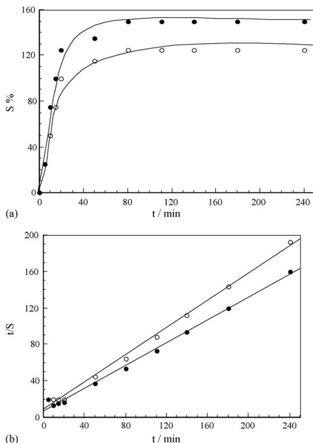
Fig. 1. Swelling (a) and second-order swelling kinetic (b) curves of beads: (●) CB-Ch-bead and (○) Ch-bead.
