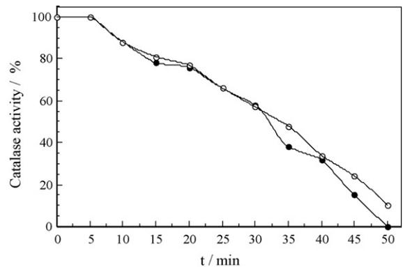
Fig. 10. Reusability of catalase: (●) CB-Ch-CAT and (○) Ch-CAT (activities were assayed at 35 °C by using 10 mM H<sub>2</sub>O<sub>2</sub> prepared in 50 mM phosphate buffer at pH 7.0).
