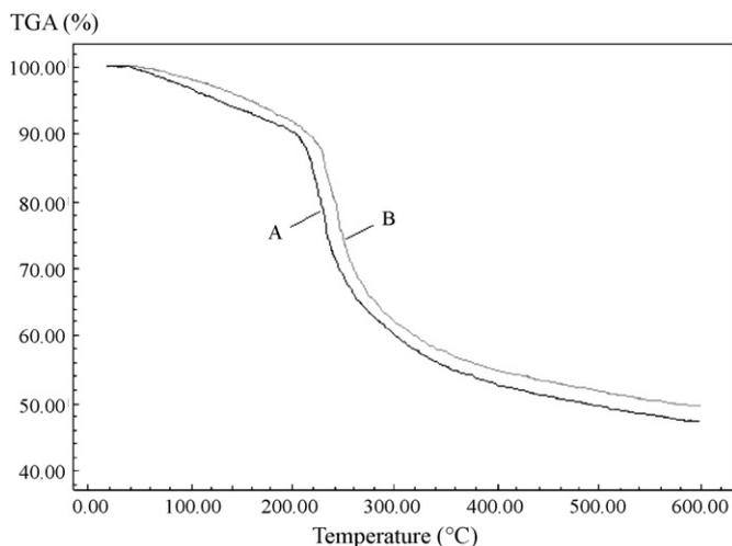
Fig. 3. TGA curves of Ch-bead (A) and CB-Ch-bead (B).
