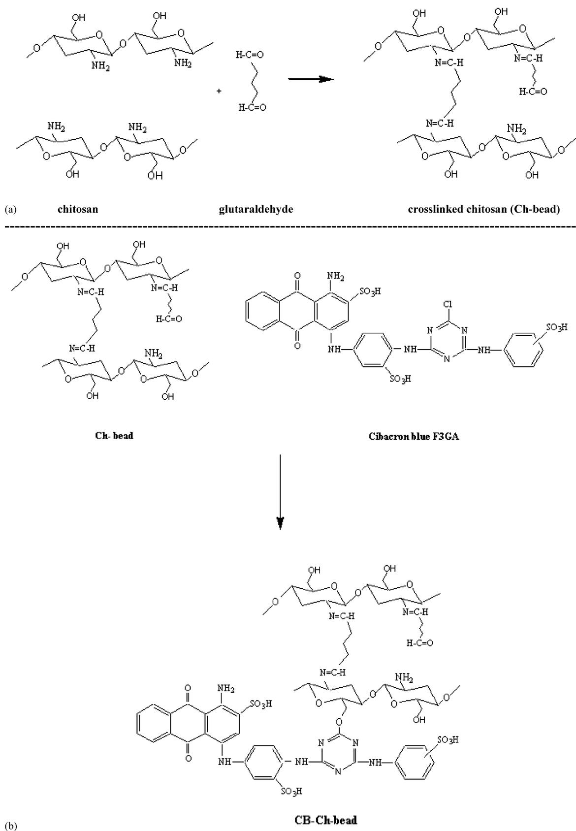
Scheme 1. Possible synthesis mechanisms of Ch-bead (a) and CB-Ch-bead (b).
