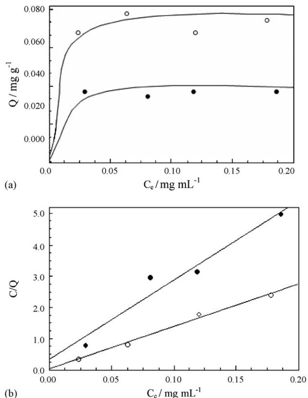
Fig. 5. The isotherms of adsorption (a) and Langmuir graph (b): (●) CB-Ch-CAT and (○) Ch-CAT.
