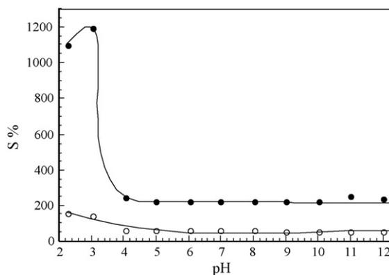
Fig. 2. The influence of pH to swelling of the beads: (●) CB-Ch-bead and (○) Ch-bead.
