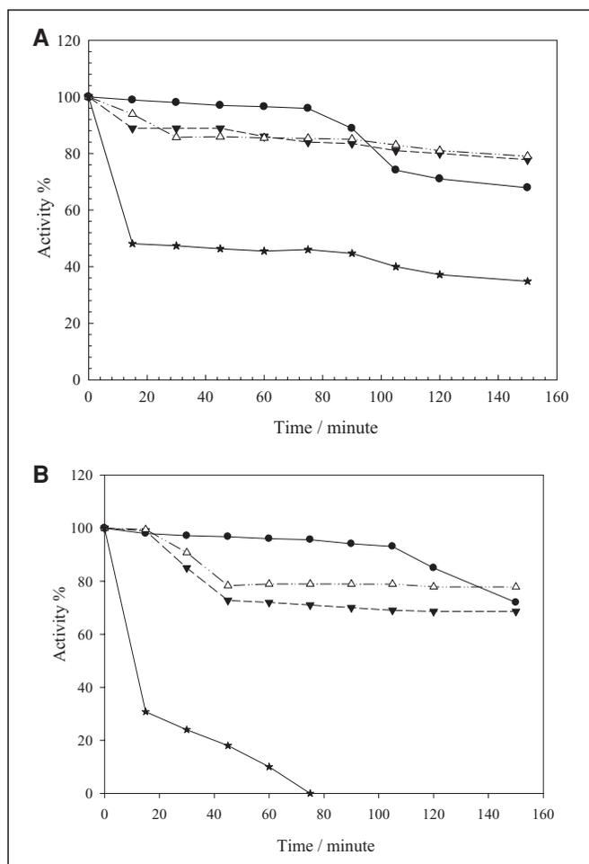
**Figure 3 – (A) Thermal stability of invertase at 50 °C. (B) Thermal stability of invertase at 70 °C. (●, PASI; ▼, PAASI; Δ, PAISI; \*, free invertase).**
