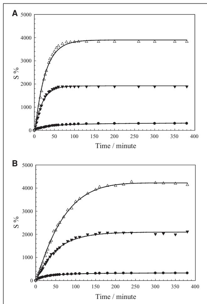
Figure 1 – Time depending swelling of the hydrogels in distilled water. (A) at 25 °C, (B) at 60 °C (●, PAS; ▼, PAAS; Δ, PAIS).
